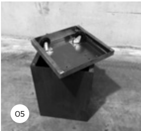
05-06: Mount both the swivel and rigid casters with the supplied nuts and bolts. The swivel casters are closer to each other than the rigid casters.
